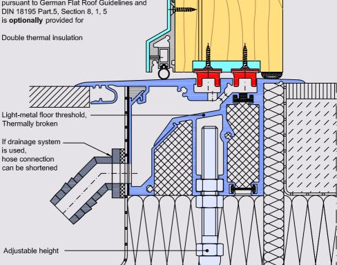
Stress group 9A pursuant to DIN 18055 Driving-rain-proof up to 100 metre floor-to-floor height (also lap-jointed doors) Assessed soundproofing measure R'Theta w=43 dB
